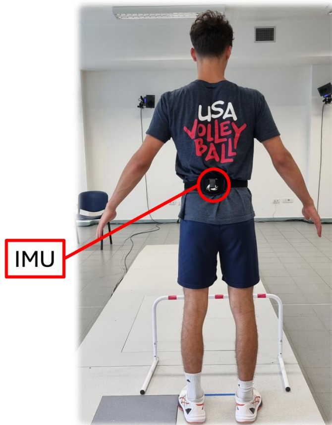
The IMU is placed at the lower back (L5/S1) via a semi elastic belt
