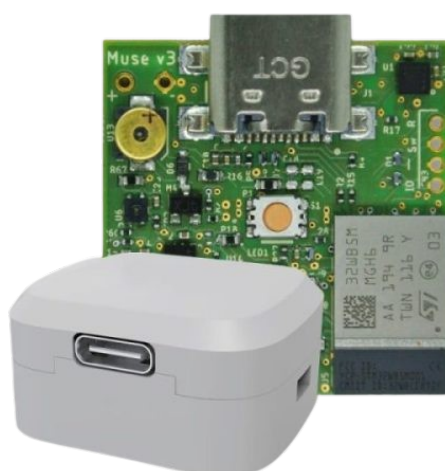
Figure 2: MuseV3 IMU sensor used in the EDATS project (source: 221e Srl)
